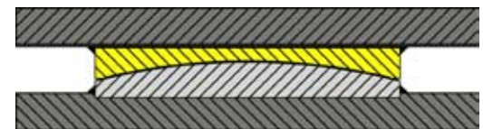
Fixed Spherical Bearings- bearings capable of multi-directional rotation and restrained from horizontal movement in any direction.
