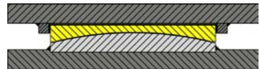
Guided Spherical Bearings- bearings capable of multi-directional rotation with sliding movement restricted to one horizontal direction.
